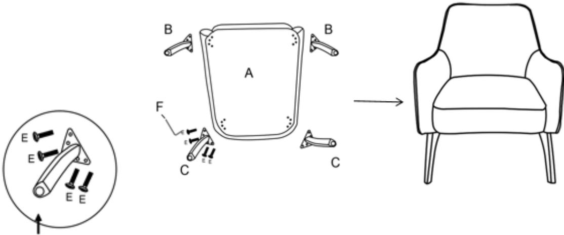
The legs can be levelled using the adjusters on the bottom of the legs
